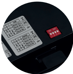
SENSOR time 15-90s range 2-8m
